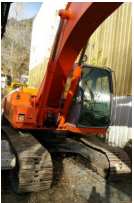
tracked excavator FIAT-HITACHI EX215
